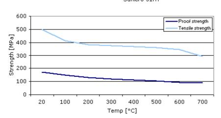
High-temperature tensile strength properties of Sanicro 31HT
